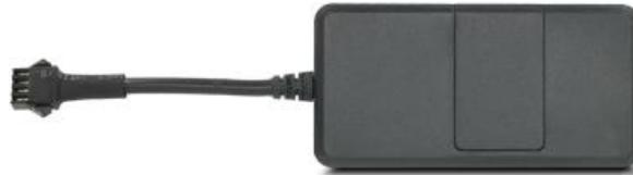
LT01 is a 4G compact GPS Tracker for vehicles, it is small in size and with internal antenna. It is designed for motorcycles, cars, vehicles and scooters, the device itself supports 9-100 volts, and it has one digital output for power off relay connecting and one digital input for ignition detect.
